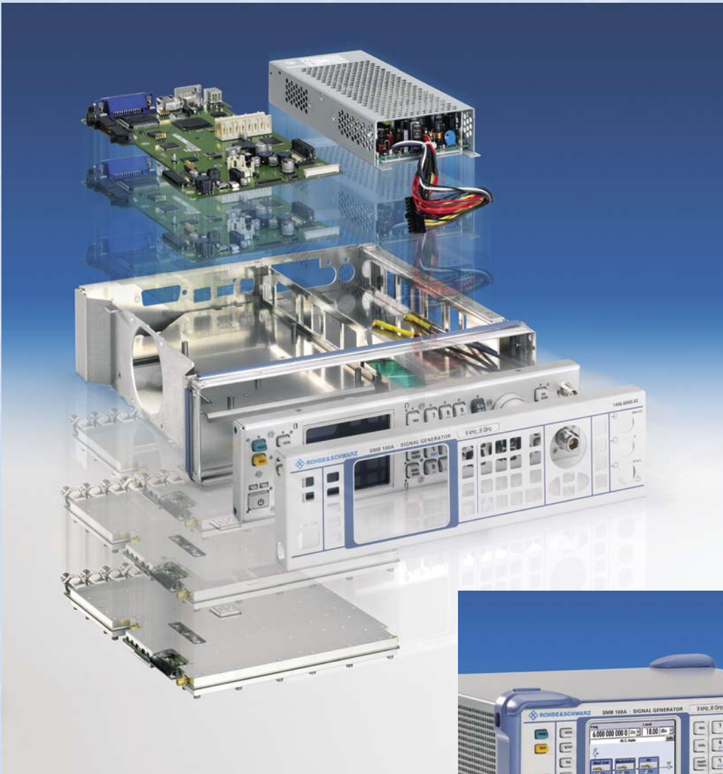
FIG 8 The R&S®SMB100A is designed for ease of service and consists of only four modules.
